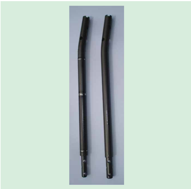
Figure 1. Photograph of tibial nails: PRECICE 1 (P1, left) and PRECICE 2 (P2, right). Note the three welds in P1 and no welds in P2.
